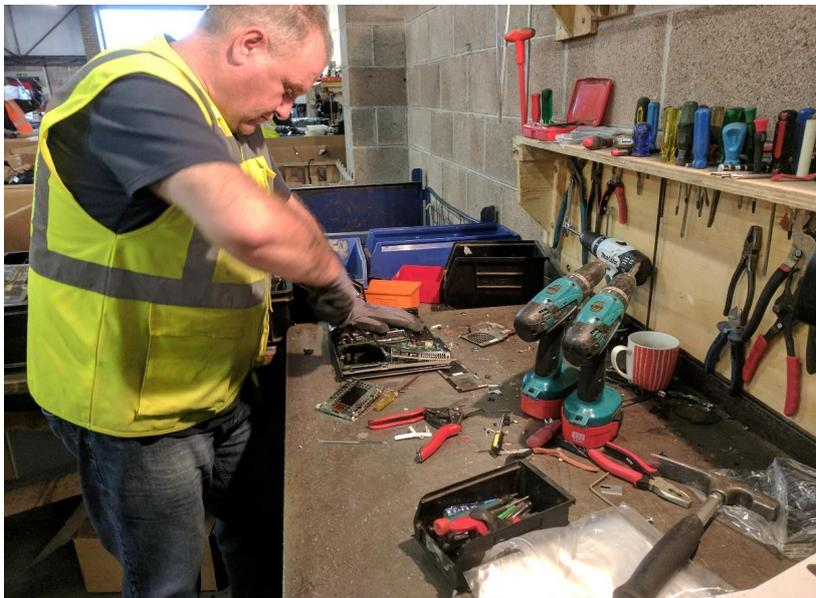
*Figure 1 - E3 Recycling operator dismantling items to recover PCBs*
