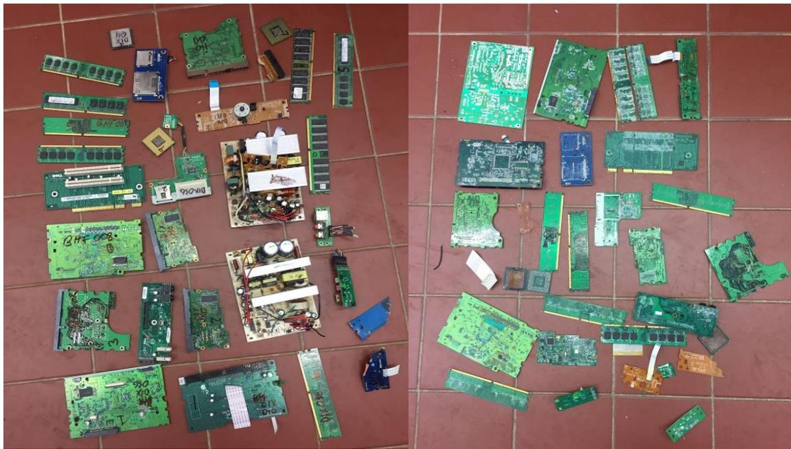
*Figure 2 - Circuit boards before (left) and after (right) depopulation (6+ year old computer towers)*
